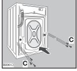
6. Fill the smaller upper hole and the two large ones with the corresponding plastic plug caps supplied in the bag containing the instruction booklet that you will find inside the drum.
